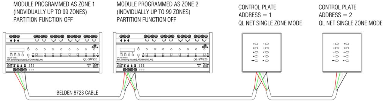
SYSTEM OPERATES IN SCENE MODE ONLY. INDIVIDUAL BUTTONS OF THE CONTROL PLATE CANNOT BE PROGRAMMED TO CONTROL INDIVIDUAL CIRCUITS ON TOGGLE ON/OFF BASIS.
