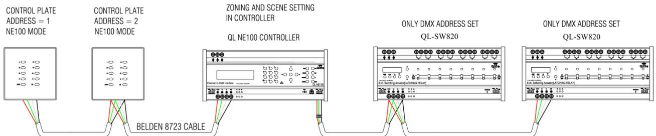
ANY BUTTON OF A CONTROL PLATE CAN BE PROGRAMMED TO OPERATE IN EITHER SCENE MODE OR TOGGLE ON/OFF MODE CONTROLLING ANY CIRCUIT/GROUP OF CIRCUITS.
