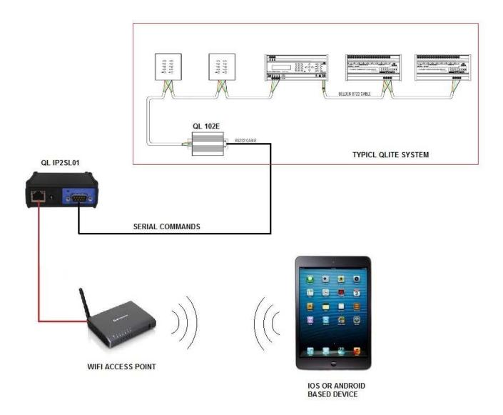
Fig 1. Module Application Diagram
