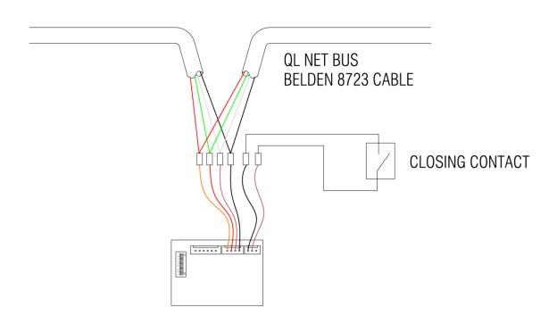
Fig 2. Module Connection
